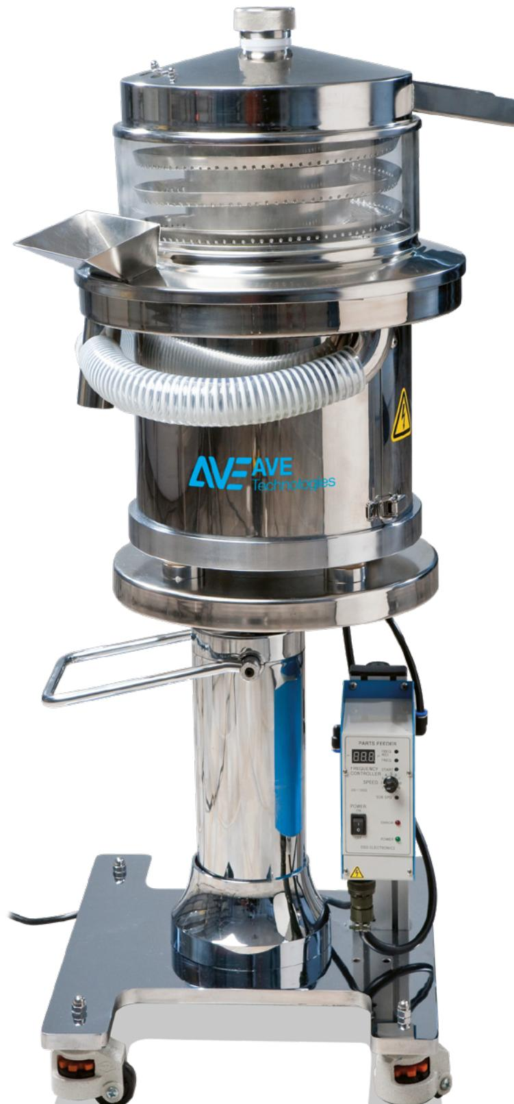
Automatic Tablet Deduster, stainless steel construction with upward product conveying designed for dedusting and deburring through vibration, compressed air and dust extraction.
